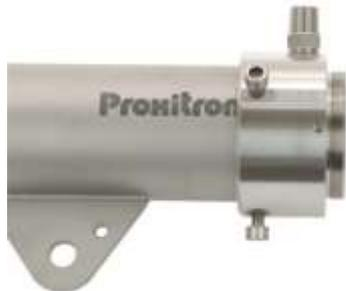
PROXITRON retro-reflective sensors can be provided with an additional air purge to protect the optics from contamination. The recommended operating pressure is 0.15 bar. This value corresponds to a consumption of 60 liters/min. The maximum operating pressure is around 0.3 bar. The scavenging air must be oil-free, dry and dust-free in order to prevent contamination of the optics. For optimum performance of the air-purge unit to use an additional protective tube OL 37 or OL 38 is recommended.
