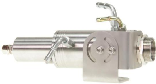
To achieve optimal alignment when using the adjustable mounting unit DAK 305, mount the optional pilot light device on the optic side of the cooling housing DAK 302. Turn on the LASER pilot light and align the beam by swiveling the cooling housing DAK 302 on the adjusting mounting unit until the light has reached the centre of the desired detection position. Fix this position by tightening the M6 screws; after alignment dismantle the pilot light device from the cooling housing DAK 302.
