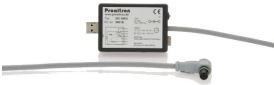
The PIROS infrared sensor needs 24 VDC voltage for parametrization. You can either feed it with the working voltage via the 8-pole S8 connector, or through the interface converter SIC 485U. In this case you will need an adapter cable ST S8 S4/5-2 to connect the interface converter to the 8-pole S8 plug on the PIROS infrared sensor and to the USB port of your PC or laptop. To make connection to your PC or laptop easier, a USB cable,
