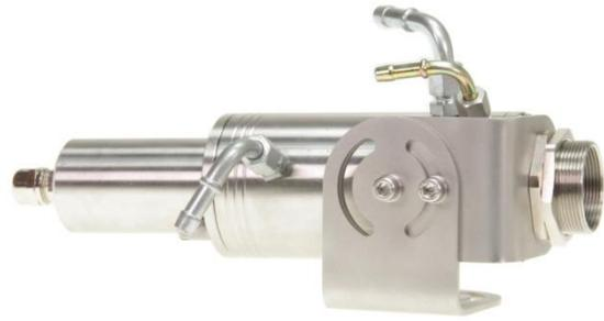
To achieve optimal alignment when using the adjustable mounting unit DAK 305, mount the optional pilot light device on the optic side of the cooling housing DAK 302. Turn on the LASER pilot light and align the beam by swiveling the cooling housing DAK 302 on the adjusting mounting unit until the light has reached the centre of the desired detection position. Fix this position by tightening the M6 screws; after alignment dismantle the pilot light device from the cooling housing DAK 302.
