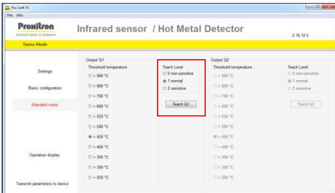
With the button **Teach Q1** and **Teach Q2** you can adjust automatically the threshold temperature to the object temperature as detected by the PIROS infrared sensor. The threshold temperature that will be set automatically via the teach procedure varies according to the Teach Level setting.
