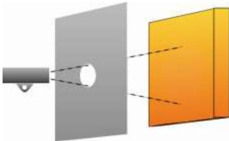
In order to exploit sensor sensitivity to the full, this opening should have a diameter of at least 50 mm. Where the object temperature is considerably higher than the threshold temperature of the sensor, a smaller opening may be chosen to increase protection.
