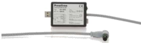
The PIROS infrared detector needs 24 VDC voltage for parametrization. You can either feed it through the 5-pole S4 connector, or through the 4-pole S6 connector being used for parametrization. To do this, connect the interface converter SIC 485U S6 and the 4-pole S6 plug on the PIROS infrared sensor; on the other side to the USB port of your PC or laptop. To make connection to your PC or laptop easier, a USB cable, length 1,5 m, is included in
