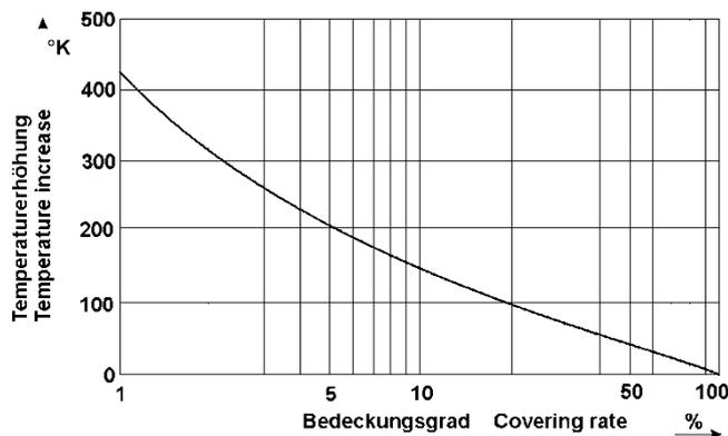
In accordance with the degree of coverage of the measuring spot by the object, the object temperature must be higher than the response temperature to enable detection.
