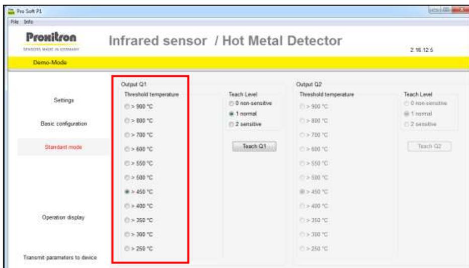
Threshold (response) temperature can be set independently for each output. Output switches if the detected object temperature exceeds the set threshold value. Output switches off when the detected object temperature falls below the set threshold value.
