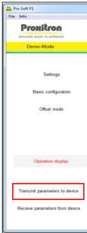
By clicking **Transmit parameters to device** settings being displayed in the software will be transferred into the sensor.
