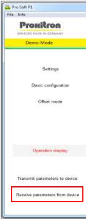
By clicking **Receive parameters from device** settings running in the equipment will be displayed in the software.
