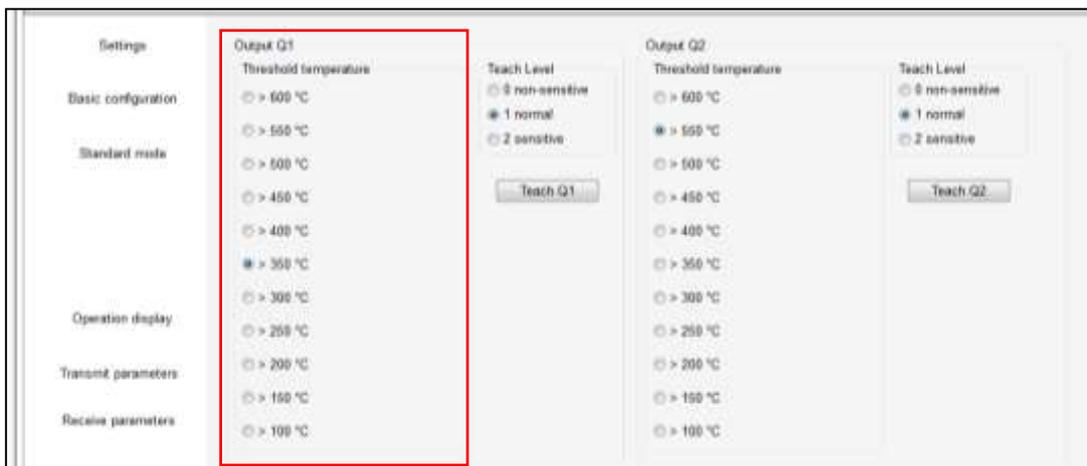
Threshold (response) temperature can be set independently for each output. Output switches if the detected object temperature exceeds the set threshold value. Output switches off when the detected object temperature falls below the set threshold value.
