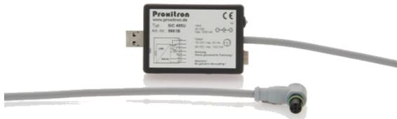
The Proxitron light barrier needs 24 VDC operating voltage for parameterization.
