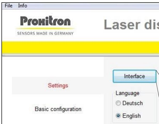
The COM port selection is different for each device, so select the appropriate interface. You normally have one choice only. Baud rate, Parity and Stop-Bits usually do not need to be set.
