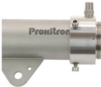
PROXITRON light barriers can be provided with an additional air purge to protect the optics from contamination. The recommended operating pressure is 0.15 bar. This value corresponds to a consumption of 60 liters/min. The maximum operating pressure is around 0.3 bar. The scavenging air must be oil-free, dry and dust-free in order to prevent contamination of the optics. For optimum performance of the air-purge unit to use an additional protective tube OL 37 or OL 38 is recommended.
