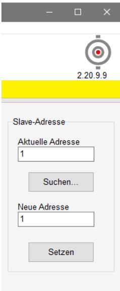
Through the slave address sensor LMA/B will be assigned a unique address, which will permit to run up to 253 sensors simultaneously on a single interface RS 485.
