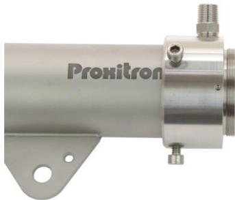
PROXITRON sensors can be provided with an additional air connection to protect the optics from contamination. The recommended operating pressure is 0,15 bar, which corresponds to a consumption of 60 l/min. The max operating pressure is around 0,3 bar. The scavenging air must be oil-free, dry and dust-free, to prevent contamination of the optic. Additional protection tube OL 46 is recommended to optimize air blow effectiveness.
