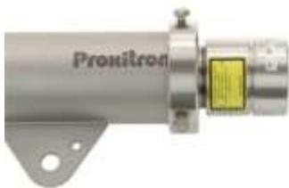
By means of the LASER Pilot Light unit DAK 308 and relevant adapter (not in the scope of supply) it is possible to align sender and receiver precisely. The spot light of the LASER pilot light approximately visualizes the middle of the optical axis.
