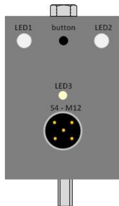
Picture 2: LED status indicators, button and connector
